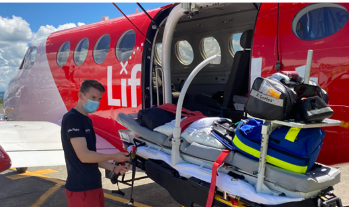
Cargo loading door of the King Air giving 1.2m clearance.
